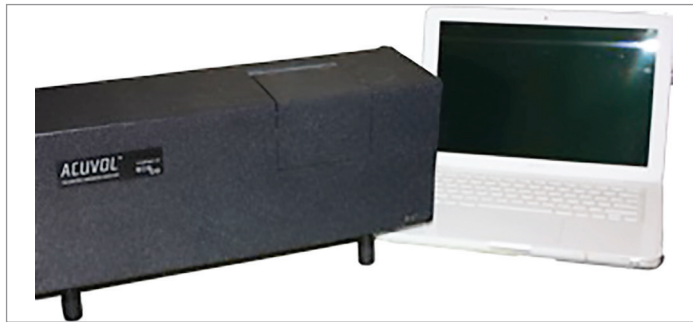
Figure 1: Set of machines for measurement of volumetric contraction and computer contained in specific software.
