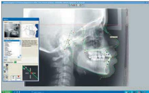
FIGURE 4 - Determining the points and performing the cephalometric tracing.
