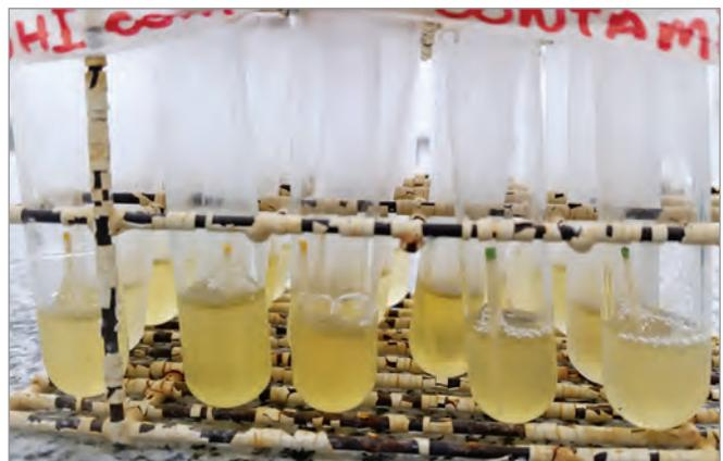
**Figure 8.** Absorbent paper points after being inserted into tubes after contamination and cultivated for 24 hours at 37 °C, being turbid, thus proving the presence of *E. faecalis*.
