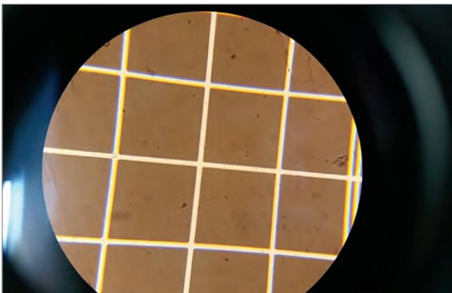
**Figure 14.** Microscopic view of the sample with *E. faecalis* in the Neubauer chamber for counting of UFC.
