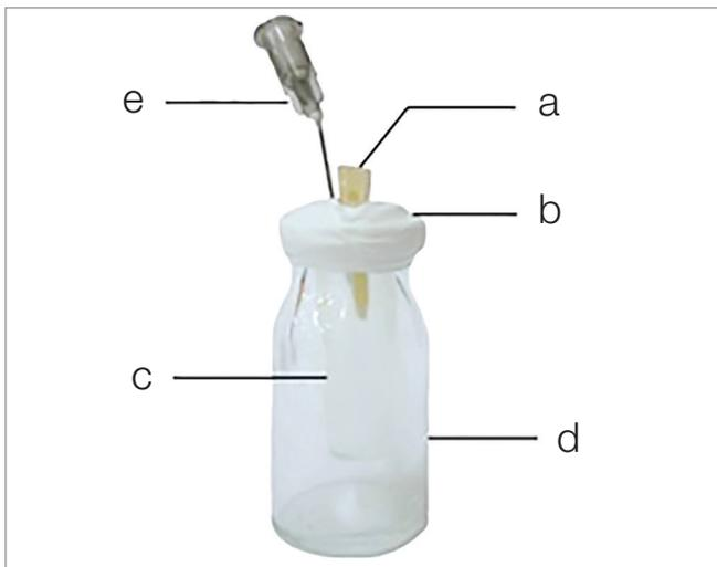
**Figure 1.** Apparatus mounted to collect debris and irrigation during endodontic treatment: **a)** tooth; **b)** thread seal tape; **c)** 2-ml Eppendorf tube; **d)** 7-ml glass vial; **e)** hypodermic needle.
