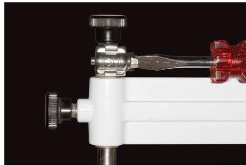
**Figure 4.** Clamp fixed at the articulator's shaft.
