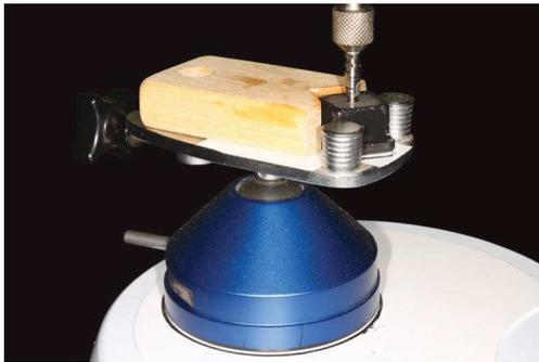
Figure 5. Implant being placed into the resin.
