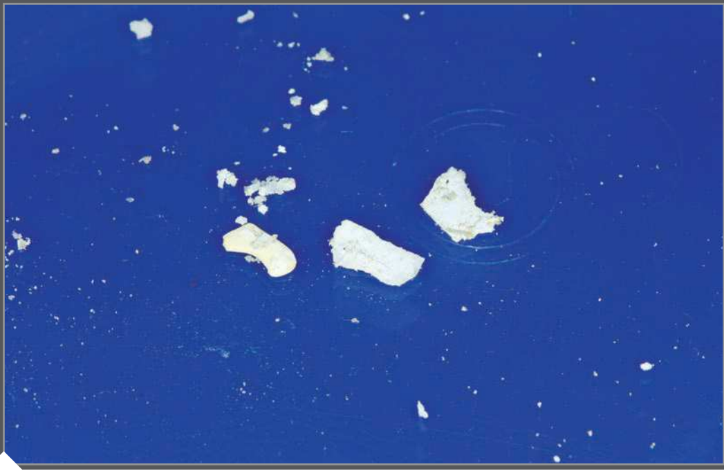
Figure 3 Calcium sulfate sample and apatite removed from SBF after 21 days of immersion.
