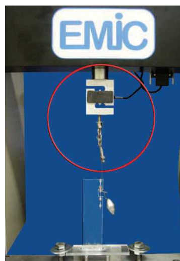
FIGURA 2 - Acrylic plate perpendicularly positioned to the ground on the grip of the testing machine.
