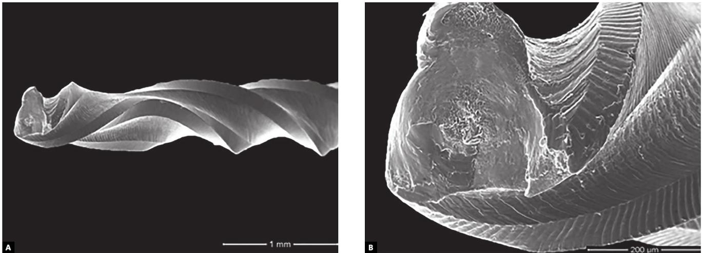
**Figure 11.** **A)** Helical shaft plastic deformation - ProTaper F4 file (100x magnification). **B)** Fracture surface and spiral reversion at fracture site (500x magnification).
