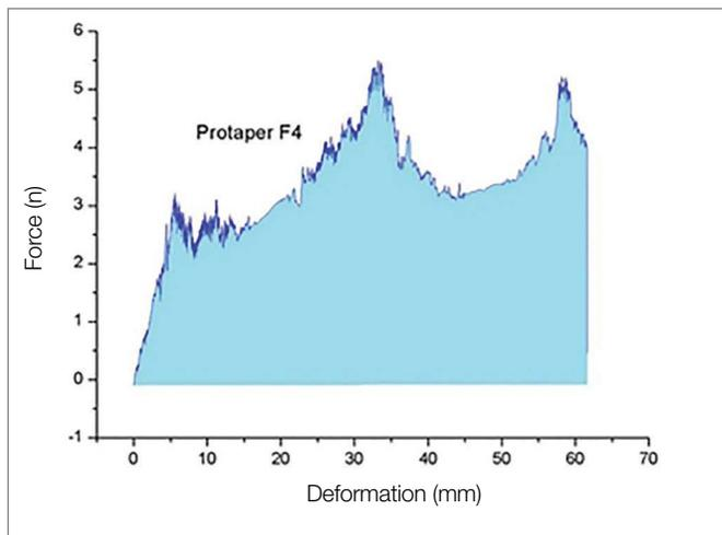
**Figure 7.** Mean toughness of ProTaper F4 files.
