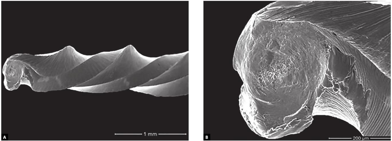
**Figure 10.** **A)** Helical shaft plastic deformation - WaveOne Large file (100x magnification). **B)** Fracture surface and spiral reversion at fracture site (500x magnification).
