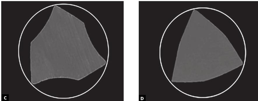
**Figure 8.** WaveOne Large file. Helical cutting shaft (A, B). Cross section of helical cutting shaft (100x magnification) (C, D).
