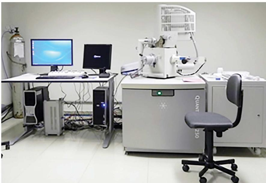
**Figure 5.** SEM unit: Quanta FEG 250.
