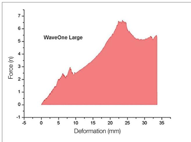
**Figure 6.** Mean toughness of WaveOne Large files.
