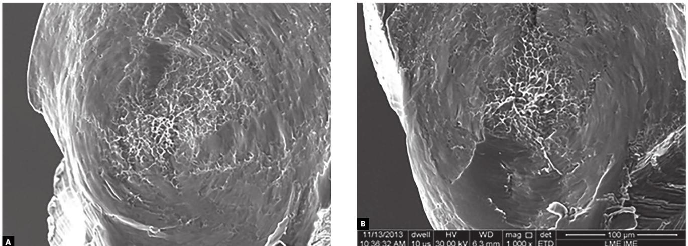
**Figure 12.** Ductile fracture surface: **A)** WaveOne Large; **B)** ProTaper F4 file (1000x magnification).
