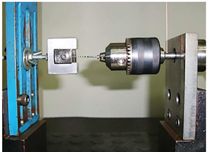
Figure 3. Photo of assembly used to apply torsional loads.
