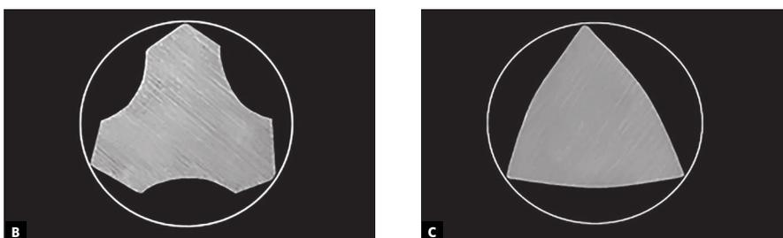
**Figure 9.** ProTaper F4 file. (A) helical cutting shaft; (B and C) cross sections along cutting shafts (100x magnification).
