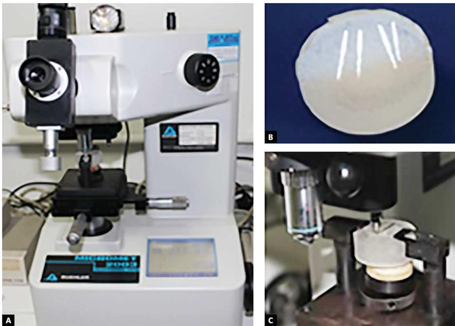
**Figure 4.** Micromet 2003 microindentation hardness tester (A) specimen embedded in resin plate (B); specimen positioning (C).
